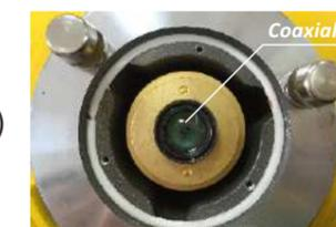
Coaxial Design of Tx/Rx Unit
